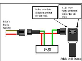
Suzuki GSXR, Hayabusa. Honda CBR. KTM, Superduke -07, RC8. (Superduke R 2008 uses Duc 749-1198 harness). RC-8 2011 and newer with 4 coils, connect green and blue coil wire pair to one cyl and yellow and brown to the other cyl.
