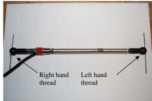
Remove orig shiftrod by opening clips at the ends. Ball joints pop off easily. Remove ball joints, one is left handed. Install ball joints on SG rod assembly and adjust to correct length. SG sensor has magic threads, can take both left and right hand bolts in the same hole.
