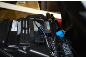
Locate black 3 wire connector behind righ hand frame rail, just below airbox. Open black connector and connect SG 3 pos connectors.
