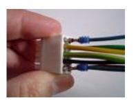
Connect the looped blue wire to killbox connector, any of the two vacant cavities are ok, then cut blue loop and pullswitch blue loop and connect together to correct length to fit your bike.
