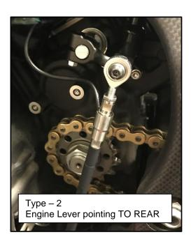
Type 1 – Voltage reduces with PUSH force – The sensor LED blinks <u>once</u> at power ON Type 2 – Voltage reduces with PULL force – The sensor LED blinks <u>twice</u> at power ON
