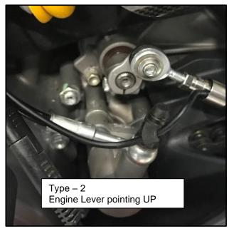
Type 1 – Voltage reduces with PUSH force – The sensor LED blinks <u>once</u> at power ON Type 2 – Voltage reduces with PULL force – The sensor LED blinks <u>twice</u> at power ON
