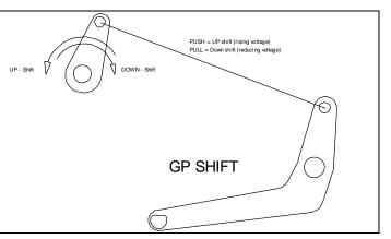
When installing the shift sensor, always try to get 90deg when the lever is resting.
