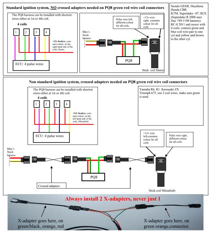
Single engs with neg pulse wire. Combine both Green and Yellow wires, cut, twist together striped Green and Striped Yellow. Do the same with solid Green and Yellow and treat as one wire and connect as above.
